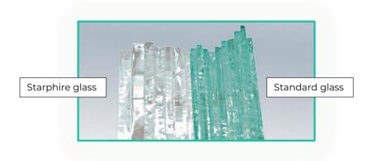
Starphire glass is a low iron glass made from silica.
